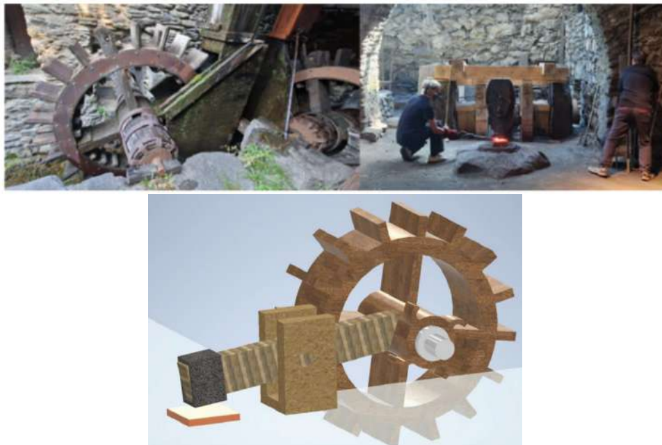
Figure 1: Farga rossell installation and simplified model used for guided mechanism identification (Source: Original)
