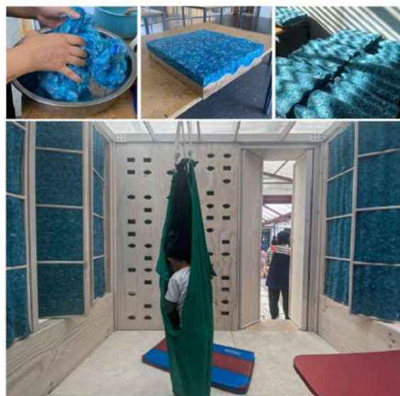
Figure 3: Top: Process of making panels with recycled textiles (2025).
