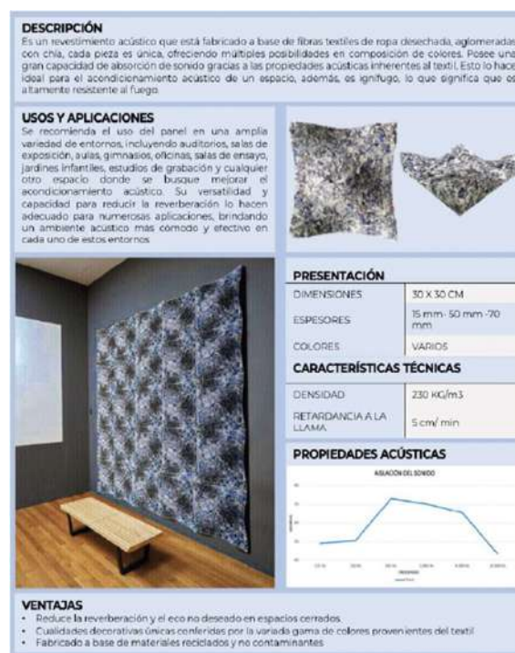
Figure 2: Panel data sheet with acoustic properties made from recycled textiles (2023).
