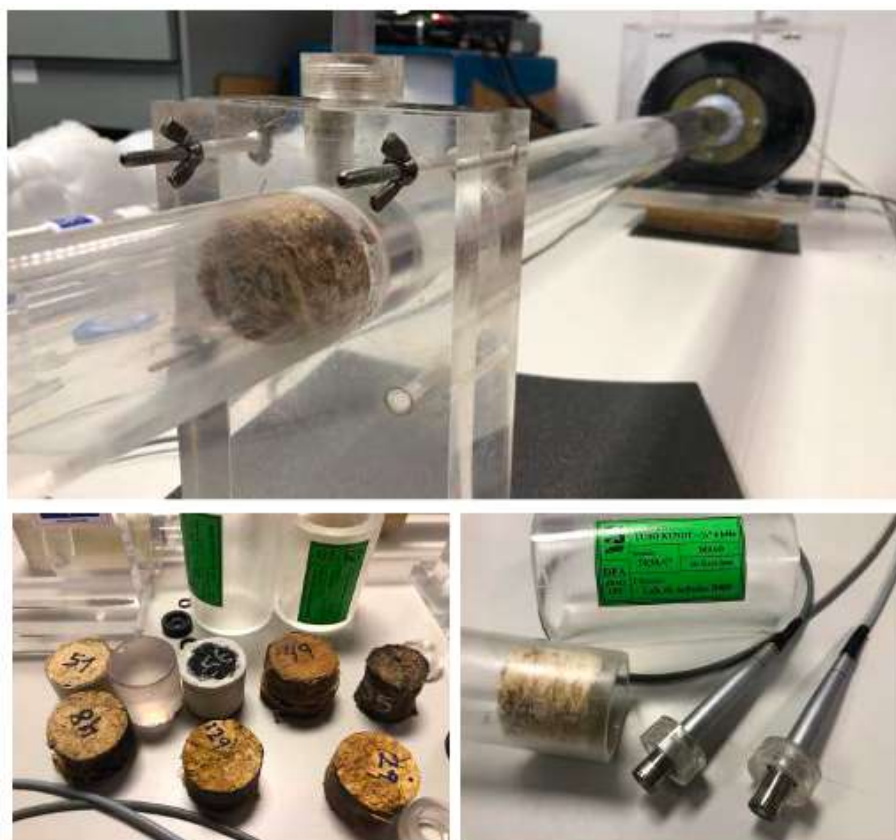
Figure 3: Kundt tube from the laboratory of the "Sonic Chrystal Technologies" research group of the UPV, Gandía.
